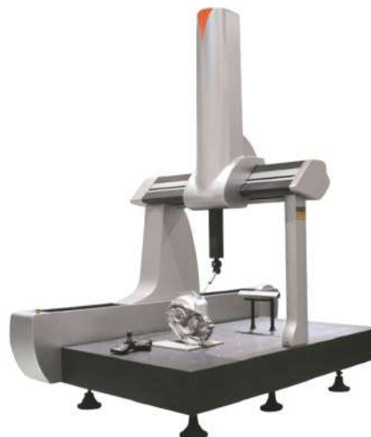
Moving Bridge Scanning Coordinate Measuring Machine Micromea 10128
